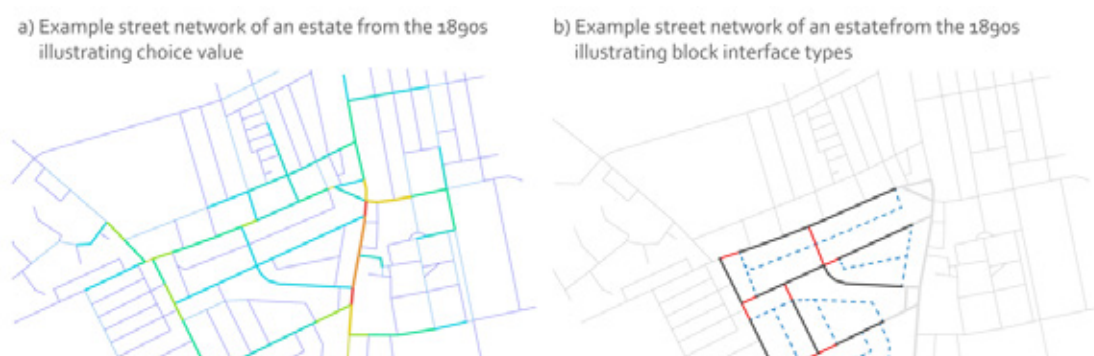
Figure 1 - Mapping comparison between through-movement potential of street networks and types of block interfaces within a 1890s estate. Diagram a) illustrates syntactic differences between street segments and shows which street is more likely to be used. Diagram b) represents four interface types observed in 1890s estates.
