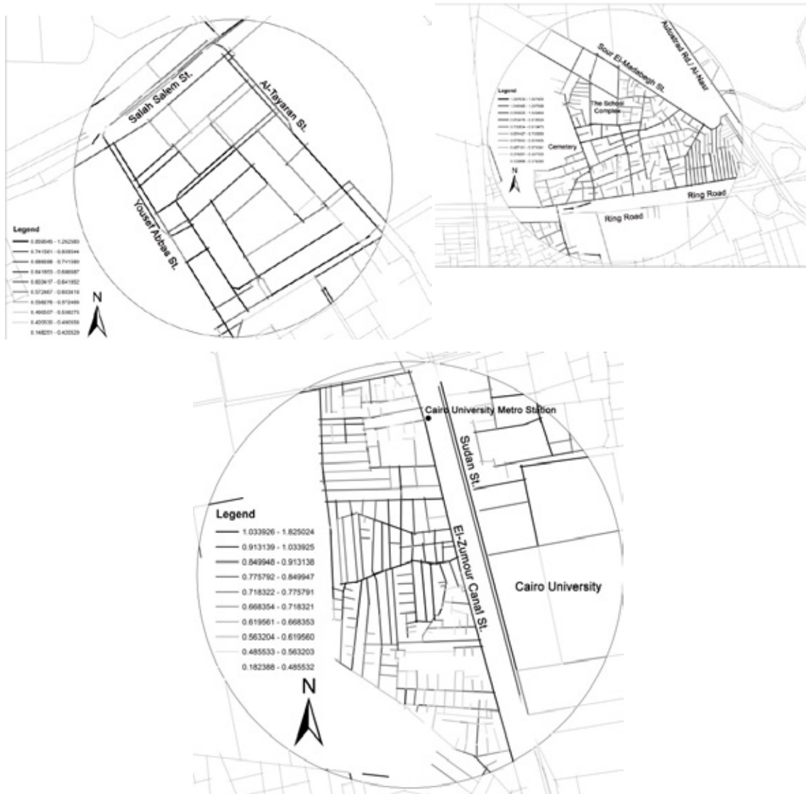
Figure 5 - Normalised angular integration R 400 in in Al-Sharekat (top left), Ezbet Al-Nasr (top right), and Abu Qatada (bottom).
