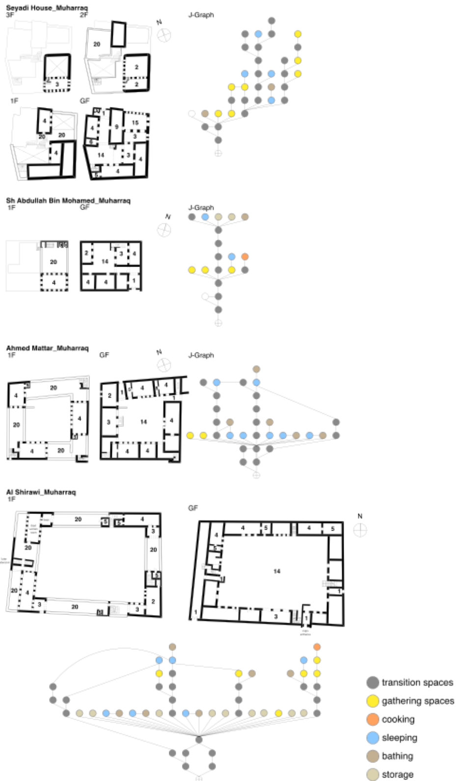
Figure 2 - Plans and J-Graphs for Traditional Bahraini Aristocratic houses. Source: Yarwood, El-Masri, 1998. 1. entrance/ vestibule; 2. majlis /reception quarters; 3. liwan /portico hall; 4. room; 5. hamman /bath; 6. kitchen/cookery/coffee burner; 7. storage; 8. door keeper; 9. men's room; 10. visitors room; 11. living room; 12. servants room; 13. animals; 14. courtyard/reception courtyard; 15. family courtyard; 16. married son courtyard; 17. servants/animals courtyard; 18. private courtyard; 19. shop; 20. Roof terrace.
