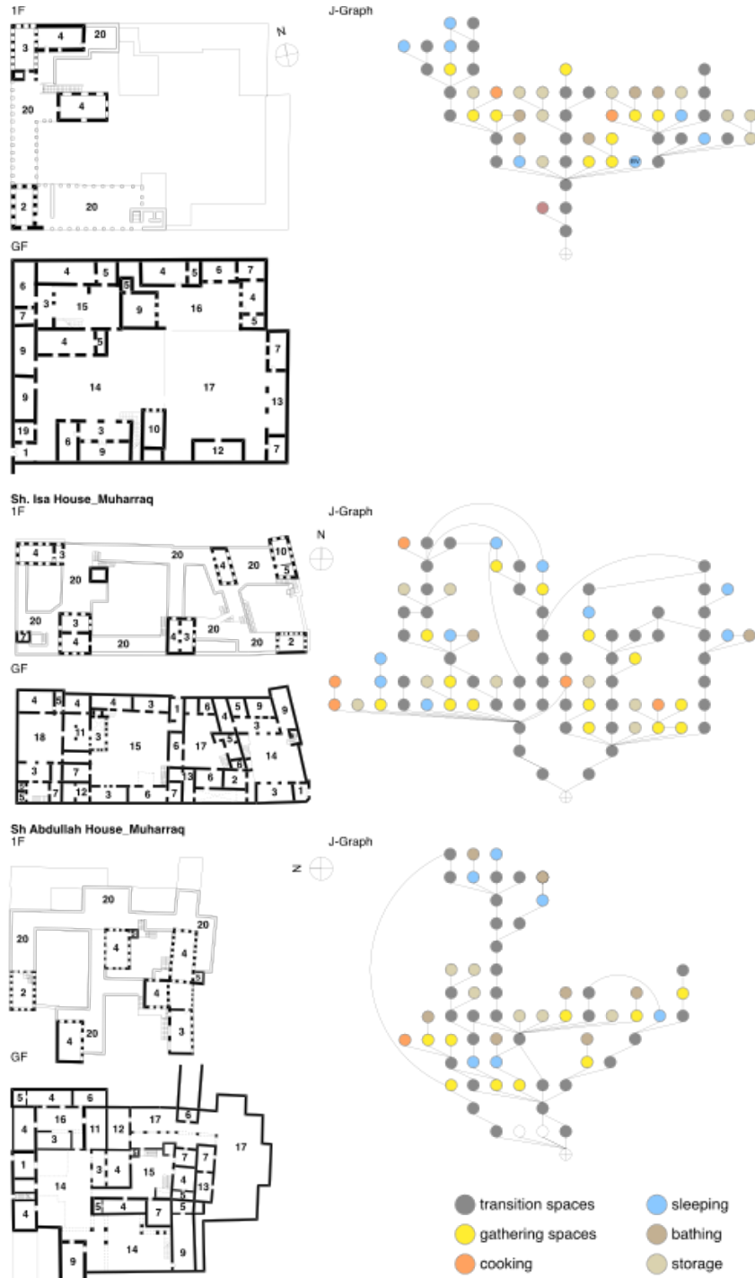
Figure 1 - Plans and J-Graphs for Traditional Bahraini Aristocratic houses. Source: Yarwood, El-Masri, 1998. 1. entrance/ vestibule; 2. majlis / reception quarters; 3. liwan /portico hall; 4. room; 5. hamman /bath; 6. kitchen/cookery/coffee burner; 7. storage; 8. door keeper; 9. men's room; 10. visitors room; 11. living room; 12. servants room; 13. animals; 14. courtyard/reception courtyard; 15. family courtyard; 16. married son courtyard; 17. servants/animals courtyard; 18. private courtyard; 19. shop; 20. roof terrace.
