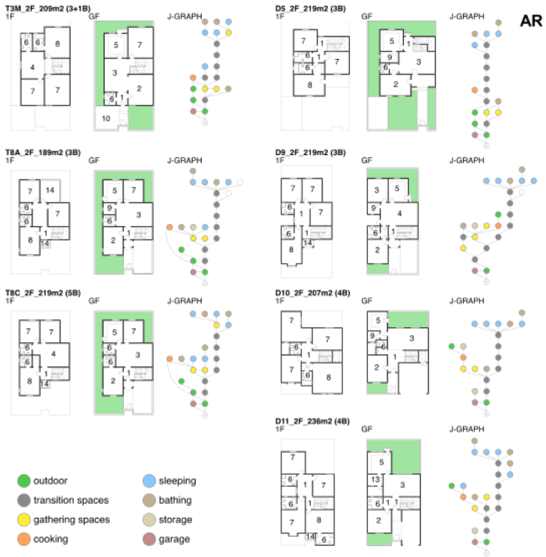
Figure 7 - Plans and J-Graphs of MOH subsidised houses — prototypes. Source: http://www.housing.gov.bh/en 1.entrance hall; 2.majlis; 3.living room; 4.family room; 5.kitchen; 6.toilet; 7.bedroom; 8.master bedroom; 9.storage; 10.garage; 11.outdoor kitchen; 12.laundry; 13.maid room. 14.veranda/terrace
