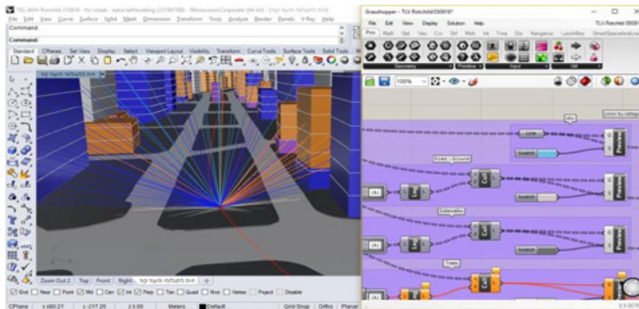
Figure 3b: Lines Of Sight coloured according to the layer (type of element) they intersect.
